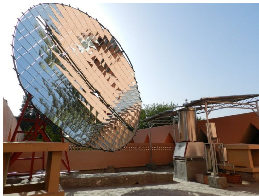
FIGURE 6.1 – Concentrateur Dish Scheffler
