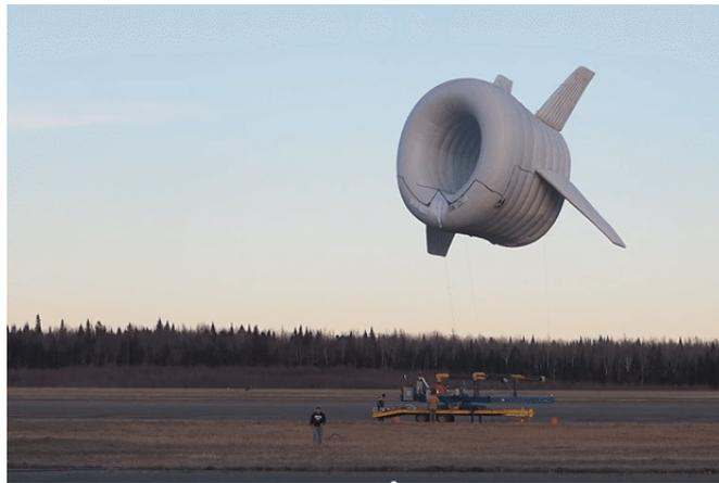
FIGURE 2.11 – Altaeros Buoyant Airbourne Turbine (Source : researchgate.net)
